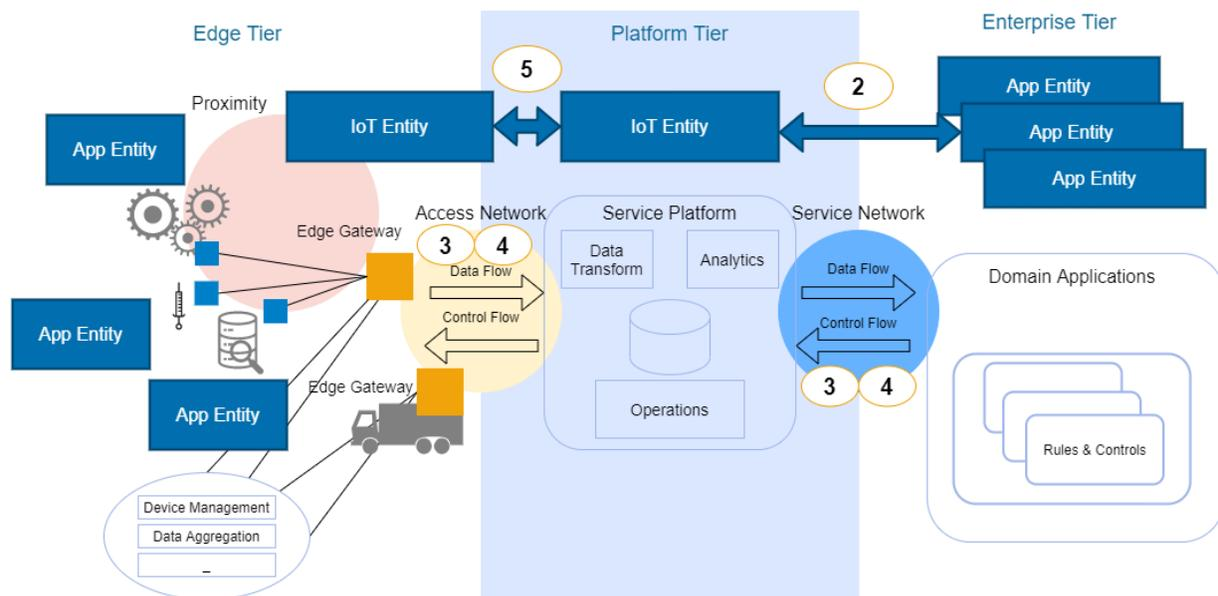
Figure 5 Open architecture of IoT by the IIRA (source [4])
