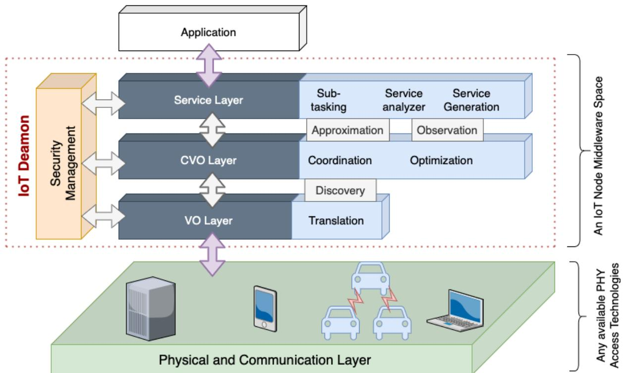
Figure 4 Service based abstraction of IoT device (source [13])
