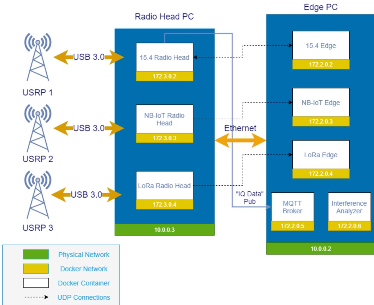
Figure 7 Coral project IoT testbed (Source [19])
