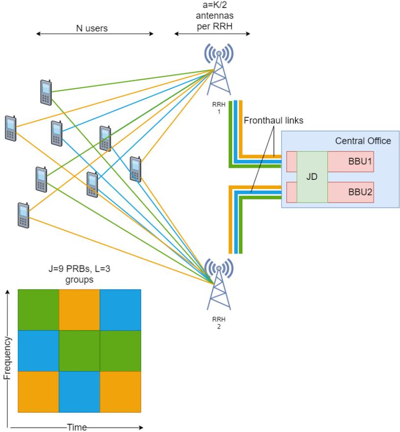
Figure 6 Uplink NOMA in C-RAN conceptual diagram (source [15])
