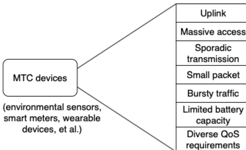
Figure 2 mMTC characteristics (source [23])
